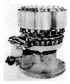
Dura-Mill Liquid Filler manufactured by Turbo Machinery Co. features a cone shaped bowl which facilitates cleaning and an antifoaming valve which prevents foaming during filling. The filling machine is available in two models; the 20 station model has filling speeds up to 300 cans per minute, the 12 station machine handles cans at the rate of 100 cans per minute. **PE2**
